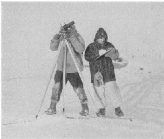
FIG. 8. Recording a pilot balloon ascent with the theodolite. (Official U. S. A. S. photo.)
