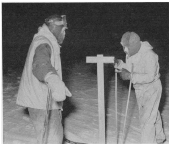
FIG. 16. One of a series of minimum thermometers being read by I. N. Schlossbach and Loran Wells on their daily round. Ten thermometers were mounted identically on exposed boards to obtain a thermal cross-section of Eleanor Bolling Valley. (Official U. S. A. S. photo.)
