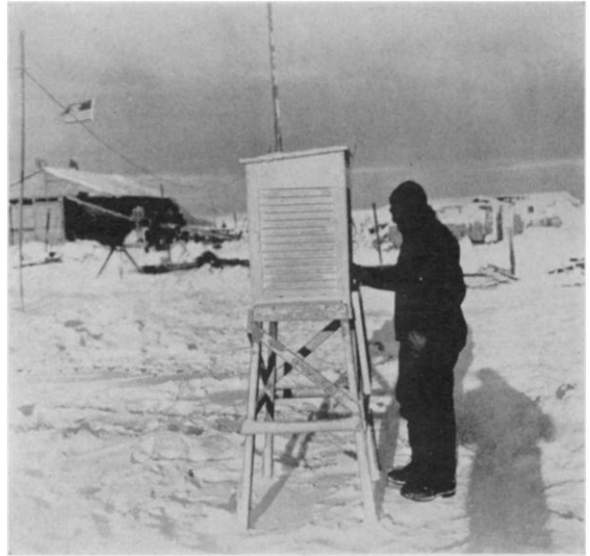
FIG. 2. Taking the observation. The shelter holds maximum, minimum, and current thermometers, and a thermograph. Temporary location, view to south; partly-completed "science building" at left. (Official U. S. A. S. photo.)
