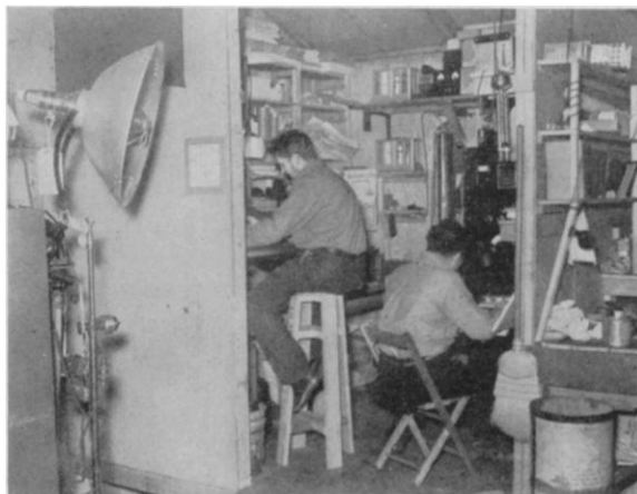
FIG. 14. Recording a radiosonde ascent. H. H. Richardson is plotting a pilot balloon ascent, while the observer is receiving and computing the radiosonde data. (Official U. S. A. S. photo.)
